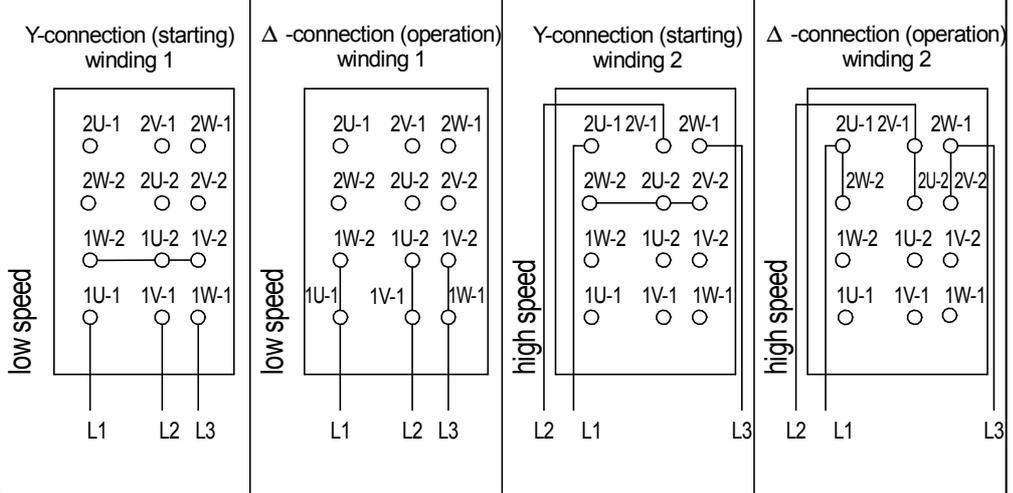
All terminals to the pole-changing switch with built-in star/delta-starting.
