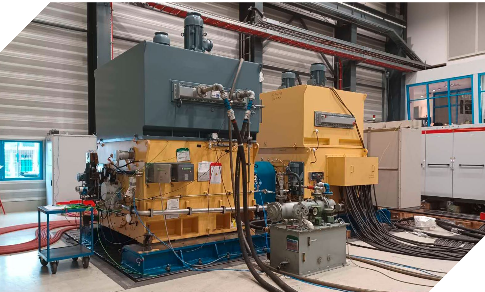
Test facility with load machine capable of 5 MW full load at 9.000 rpm
